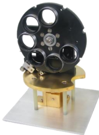
Figure 1. Example filter wheel assembly controlled by motor with position feedback from mechanical switches
