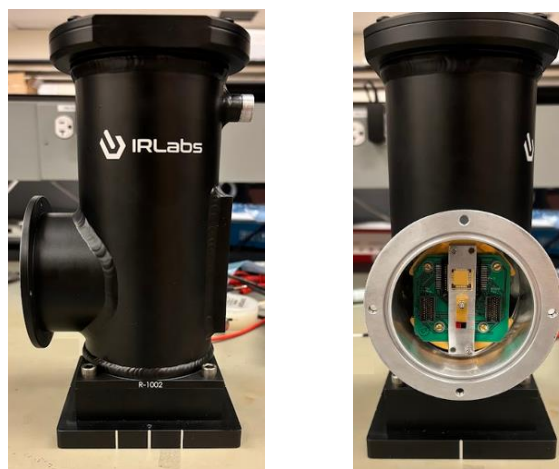
Fig. 1. Rigel dewar from I.R. Labs in Tucson AZ. The side profile of the dewar shows how compact it is as well as some location calibration marks. The front view (right side of picture) shows the cold finger as well as the temperature sensor.
