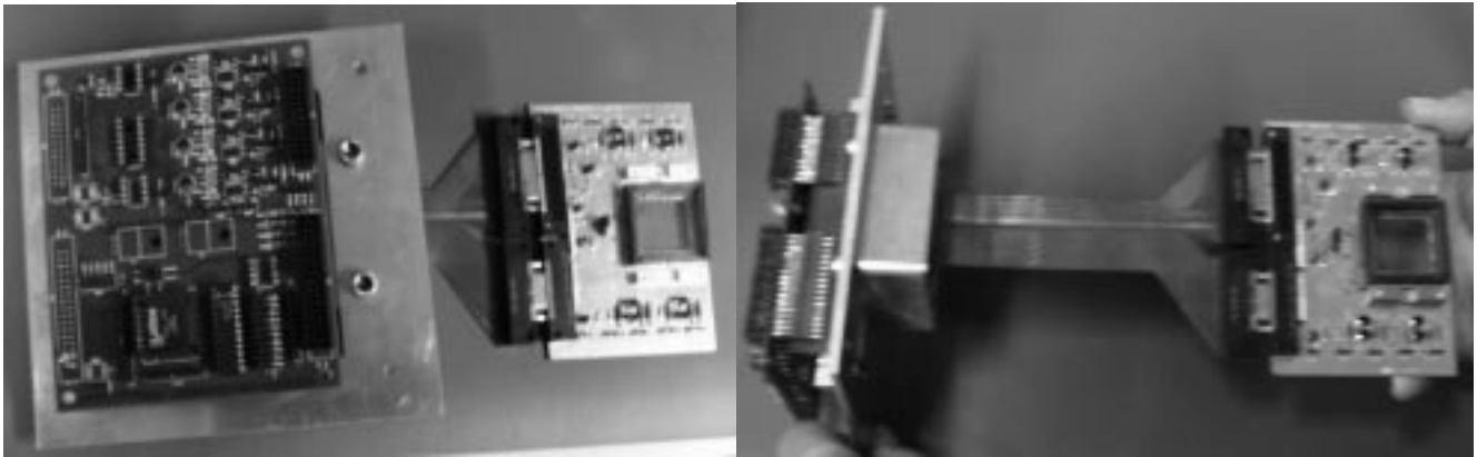
Figure 6. Preamp. Pictures show the preamp board on the left connected via flex circuit to the FPA fanout board, illustrating the short electrical path length. The entire physical interface from the FPA to the preamp can be removed from the dewar for test and development. The 4-channel preamp circuit occupies the top half of the PCB, while the clock pattern generator FPGA and driver IC with series wave-shaping resistor occupies the lower half of the PCB.
